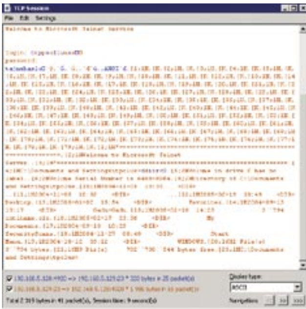
Fig. 5. Intercepted user password and a fragment of a Telnet protocol session from the intruder's point of view.
