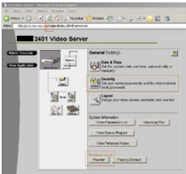
Fig. 2. Screenshot of the administrating panel of a network camera, illustrating a vulnerability which was discovered in 2003 and promptly eliminated by its maker. It was found that it could have been accessed without logging on, by adding a slash in a network address. The options, then accessible from the screen, are marked: the possibility to manage user accounts and to reset the device.
